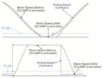
1: The command source is register. ZCLAMP function will use the register with acceleration / deceleration processing to judge if this function is enabled. When ZCLAMP conditions are established, the motor speed will be set to 0.
