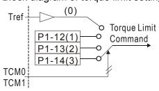
When desiring to use torque limit function, users could use parameter to set this value to 1 and limit the torque for good. Thus, the user can save one DI setting. Also, users could enable or disable the limit function via DI.TRQLM, which is a more flexible way but would need to take one DI setting. Torque limit can be enabled by P1-02 or DI.
