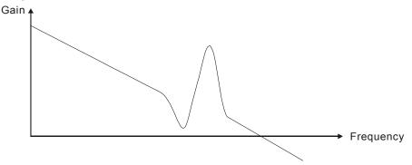
When the value of P2-25 is increased from 0, BW becomes smaller (See as the following diagram). Although it solves the problem of resonance frequency, the response bandwidth and phase margin is reduced.
