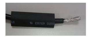
(1) Cut through the cable and expose the core wire which covers the metal core wires with shielding. The reserved core wire length should be 20~30mm. Then, cover a 45mm heat shrink tube on the cable.
