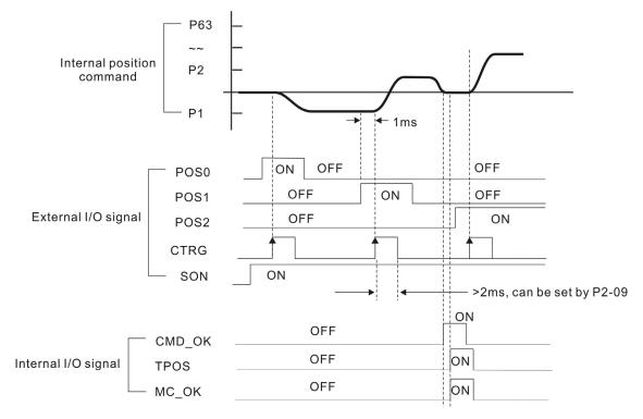
$\mathsf{CMD}\_\mathsf{OK}$  :  $\mathsf{CMD}\_\mathsf{OK}$  is activated when the servo drive has detected that  $\mathsf{Pr}$  command has been completed
