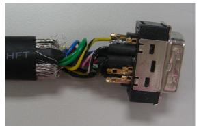
(3) Leave a length of 5~10mm metal core wires with shielding outside of the cable. The length is about the width of the metal saddle. The other unexposed wires of the cable should be protected by heat shrink tube for good ground contact.
