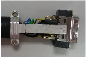
(4) Install a metal saddle to fix the exposed metal core wires. The metal saddle must completely cover all the exposed metal core wires. The extended sheet metal should be connected to the metal part of the connector.
