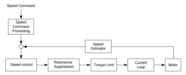
The speed command unit is to select speed command source according to Section 6.3.1, including the scaling (P1-40) setting and S-curve setting. The speed control unit manages the gain parameters of the servo drive and calculates the current command for servo motor in time. The resonance suppression unit is to suppress the resonance of mechanism. Detailed descriptions are shown as the following:
