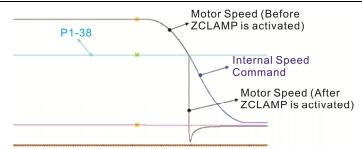
1: The command source is analog speed command. ZCLAMP function will use the analog speed command without acceleration / deceleration processing to judge if this function is enabled. When ZCALMP conditions are established, the motor speed decelerates to 0 through S-curve. If not, the motor follow the analog speed command through S-curve.
