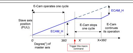
Refer to the figure below, triggering this macro command, E-Cam will stop for one cycle regardless the degree (X) where E-Cam is.
