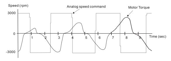
Analog speed command filter smooth the analog input command. Its time program is the same as S-curve filter in normal speed. Also, the speed curve and the acceleration curve are both continuous. The above is the diagram of analog speed command filter. The slope of speed command in acceleration and deceleration is different. Users could adjust the time setting (P1-34, P1-35 and P1-36) according to the actual situation to improve the performance.
