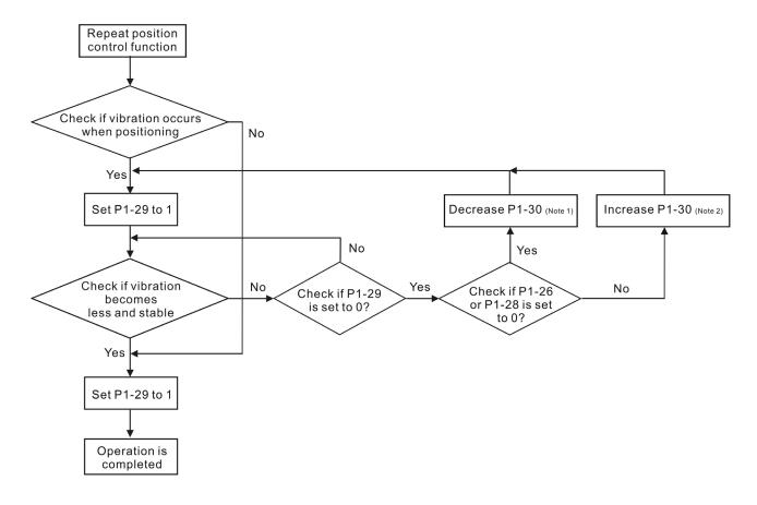
Note 1: When the value of P1-26 and P1-28 is 0, it means it is unable to search the frequency. It is probably because the detection level is set too high and is unable to detect the low-frequency vibration.
