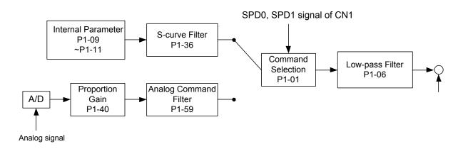
The upper path is the command from register while the lower one is external analog command. The command is selected according to the status of SPD0, SPD1 and P1-01(S or Sz). Usually, Scurve and low-pass filter are applied for having a smooth resonance of command.
