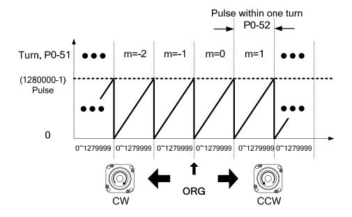
Figure 12.1 Pulse counting in absolute coordinate system
