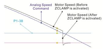
0: The command source is register. ZCLAMP function will use the register speed command with acceleration / deceleration processing to judge if this function is enabled. The motor will be locked at the position where ZCALMP conditions are established.
