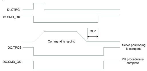
Description of command triggered method in PR mode:
