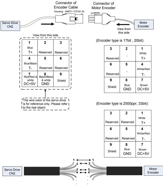
If not using housing and directly wire the cores, please follow the corresponding core number for wiring. For example, core number 1 from the servo drive CN2 should connect to core number 1 from the motor encoder; core number 2 from the servo drive CN2 should connect to core number 2 from the motor encoder and so on. Please number the cores from the servo drive in order and then connect it to the encoder.
