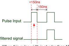
When this pulse width is shorter than 150 ns, it will be seen as low level. Two input pulse will be seen as one.
