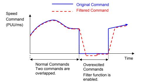
Note: When this filter function is enabled, it may cause the motor goes beyond the original position. Usually, the motor will return to the original position after the command becomes stable. However, if the command does not become stable, the internal position errors may be accumulated and result in AL.404.
