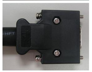
(6) Tighten the screws to complete a shielded CN2 connector.
