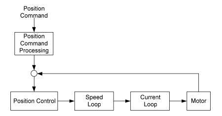
For a better control, the pulse signal should be processed and modified through position command unit. Structure is shown as the diagram below.
