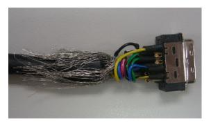
(2) Spread the metal core wires with shielding and turn it upside down in downward direction. Ensure to follow the above table of CN2 Terminal Signal Identification to connect the pins one by one.
