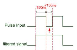
When this pulse width is shorter than 150 ns, it will be seen as high level. Two input pulse will be seen as one.
