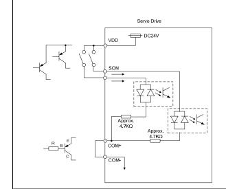
C12: The wiring of DI. The servo drive applies to the external power.
