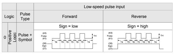
For digital circuit, it uses 0 and 1 represents two status, which is high voltage and low voltage. In Positive Logic, 1 represents high voltage and 0 represents low voltage and vice versa in Negative Logic.
