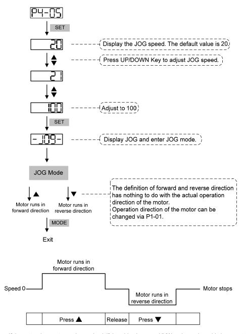
If the motor does not run, please check if the wiring between UVW and encoder cable is correct. If the motor run abnormally, please check if the UVW phase sequence is correct.
