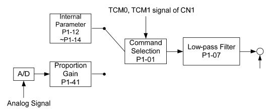
The upper path is the command from register while the lower one is external analog command. The command is selected according to the status of TCM0, TCM1 and P1-01 (T or Tz). The torque represented by analog voltage command can be adjusted via the scaling and can obtain a smoother response via low-pass filter.
