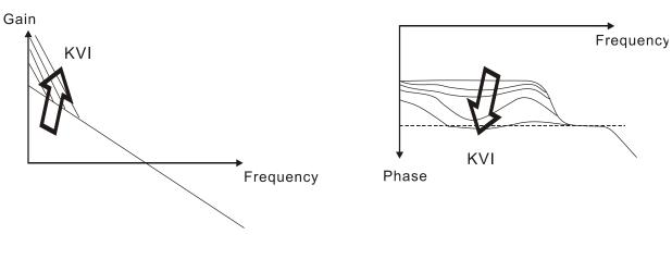
STEP 3: Select the value of KVI, if the value of phase margin is too small, re-adjust the value of KVP again to obtain the value, 45deg of phase margin.
