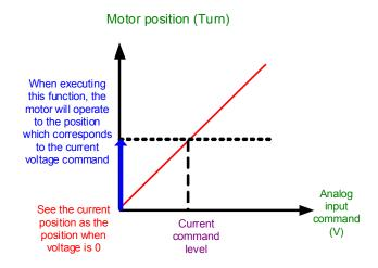
1: After SERVO ON, if the command level is not changed, the motor will not operate. The position the motor stops is the position that corresponds to the current command level.
