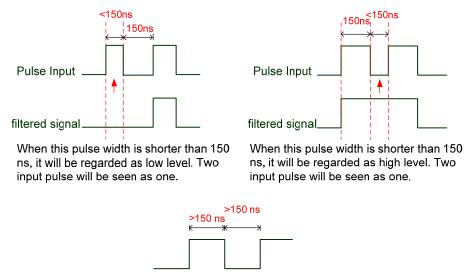
When High, Low duty of the pulse width are longer than 150 ns, it can ensure the pulse command will not be filtered.
