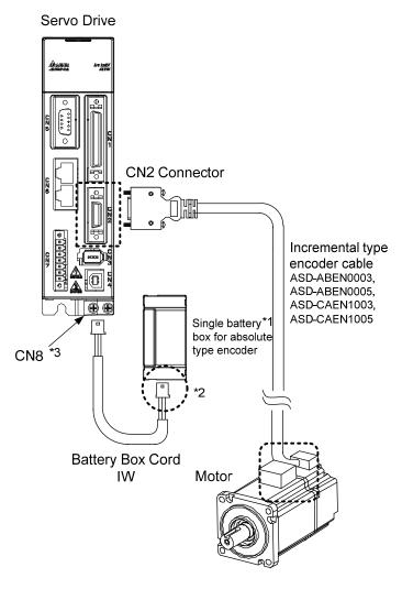
NOTE This is the wiring diagram for connecting to a single battery box. The scale of the objects does not match the dimensions as shown in the drawing above. For different models of AC servo drives and motors, the connection cables may differ.
