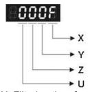
X: Filtering time for 1st monitoring variable
