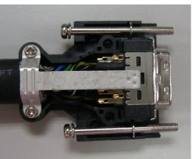
(5) Install the connector with shielding into the plastic case as shown in the figure.
