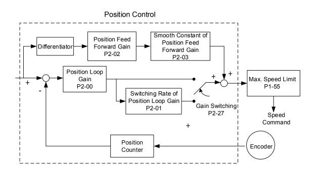
When the value of proportional gain, KPP is set too big, the response bandwidth of position loop will be increased and diminish the phase margin. And the motor rotor rotates vibrantly in forward and reverse direction at the moment. Thus, KPP has to be decreased until the rotor stops vibrating. When the external torque interrupts, the over-low KPP cannot meet the demand of position deviation. In this situation, parameter P2-02 can effectively reduce the position error.
