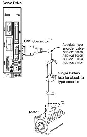
NOTE This is the wiring diagram for connecting to a single battery box. The scale of the objects does not match the dimensions as shown in the drawing above. For different models of AC servo drives and motors, the connection cables may differ.
