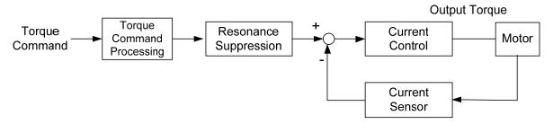
The torque command unit is to select torque command source according to Section 6.4.1, including the scaling (P1-41) setting and S-curve setting. The current control unit manages the gain parameters of the servo drive and calculates the current for servo motor in time. Since the current control unit is very complicated, and is not relevant to the application. There is no need to adjust parameters. Only command end setting is provided.
