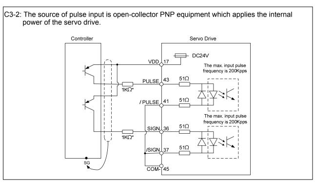
NOTE Resistor of  $1K\Omega(1w)$  has to be connected.
