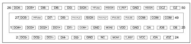
The rear wiring terminal of CN1 connector
